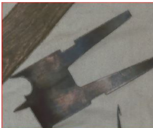
One style of Oliver's handmade auger bits. The circle cutter is next to the round cutout, opposite the flat cutting edge.
