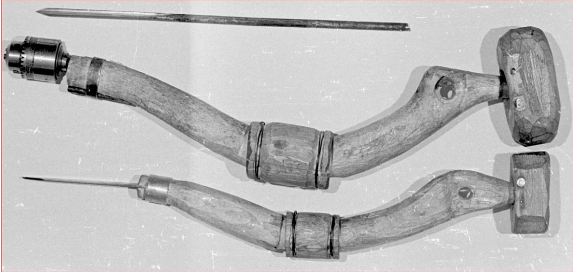
Note the two-piece hand grips and top handles, all of which turn. Images: Curt Madison
